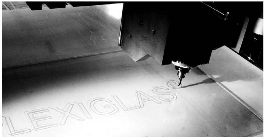
Fig. 27: Engraving with CNC portal-type machine; single-fluted graving bit.
