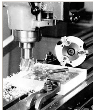
Fig. 24: Routing of PLEXIGLAS® with shell endmill; various other cutter types: (a) double-fluted cutter; (b) cylindrical cutter; (c) diamond cutter
