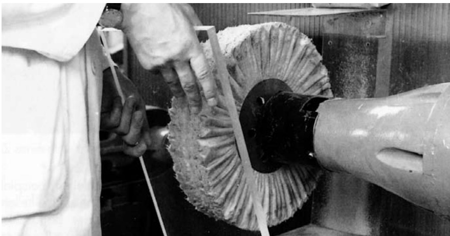
Fig. 40: Polishing against a cloth buffing wheel
