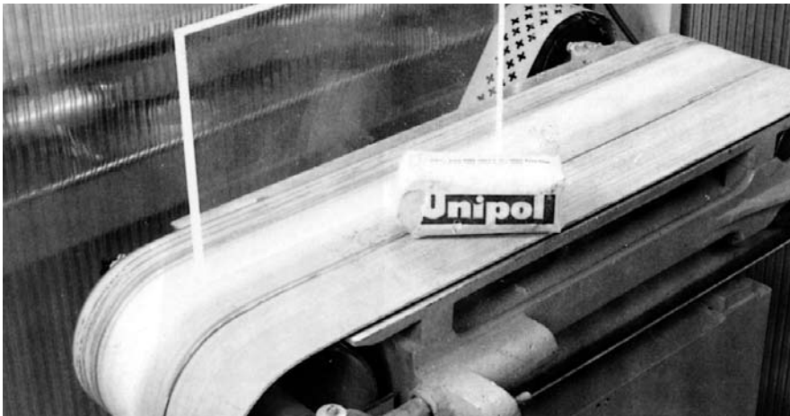
Fig. 39: Polishing against a felt belt
