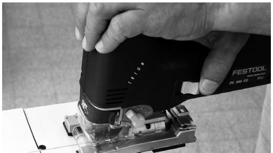
Fig. 10: Jigsawing after predrilling
