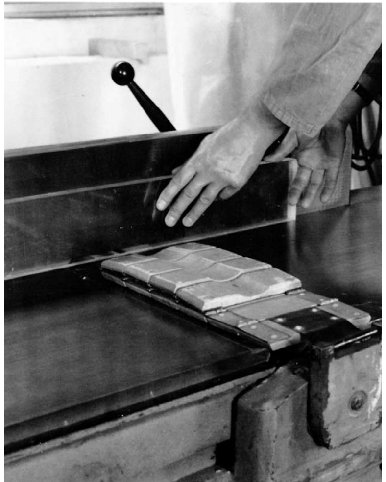
Fig. 36: Smoothing the edges with a surface planer
